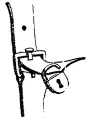
*Rings.*—In packing-gear and other harness, use is frequently made of rings. Iron ones may be replaced by a loop of tough wood, such as the peasants of the Campagna commonly employ: a piece of the thickness of a small walking-stick, and eight inches long, is bent (see "Wood, to bend"); its arms are notched when they cross, and are firmly nailed or lashed.
