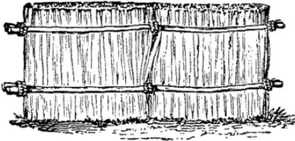
reeds, or herbage, of almost any description, is simply nipped between two pairs of long sticks, which are respectively tied together at their ends, and at a
