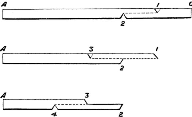
Let A O be the log. Cut two notches (1), (2), on opposite sides. Hold the log by the end A, and strike the end violently against the ground; the piece O, 1, 2, will fly off. Then make the cut (3) on the side opposite to (2), and again strike, and the piece 1, 2, 3, will fly off. So again with cut (4), &c. (Peal.)
