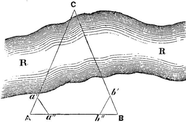
obtained for determining the lines  $AC$  and  $BC$ . The problem can be worked out, either by calculation or by protraction. I have made numerous measurements in this way, and find the practical error to be within five per cent.
