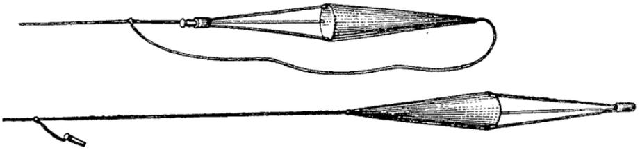
When the peg is drawn out by the usual jerk, the bag no longer presents its mouth to the water, but is easily drawn in by the line attached to its point.
