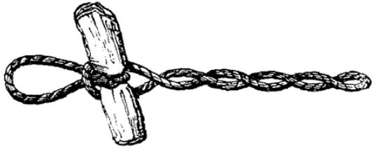
of a buckle breaks, a nail or a peg, pushed through the buckle-hole, as in the figure below, will replace it.
