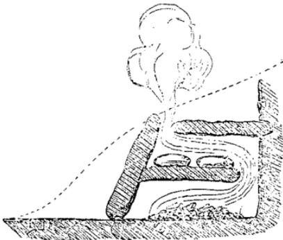
and two flat stones are slid horizontally, like shelves, into grooves made in the sides of the hole, as shown in the figure; where it will be observed that the uppermost stone does not quite reach to the face of the bank, and that the lowermost stone does not quite reach to the back of the
