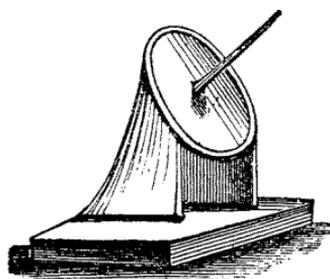
The figure represents the well-known equinoctial sun-dial. It can easily be cast in lead. The spike points towards the elevated pole, and
